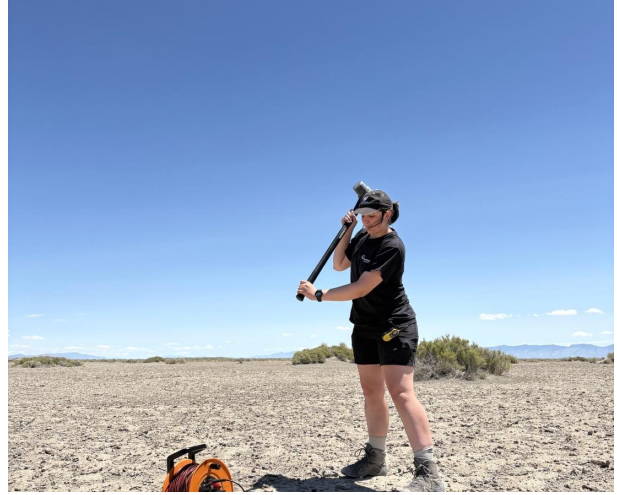
EarthScope RESESS intern Bella Chuchro performs a controlled hammer-source test for geophysical data acquisition.
