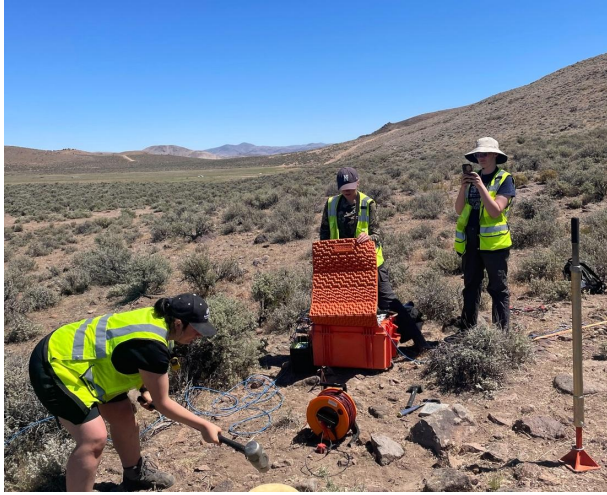
A field team prepares equipment and conducts an active-source measurement.
