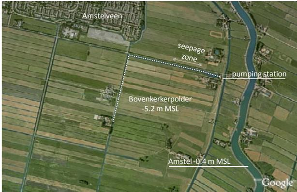
Fig. 3 DTS set-up in the Bovenkerkerpolder
